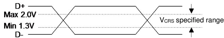
\*5: They indicate rising time ( $T_{rise}$ ) and falling time ( $T_{fall}$ ) of the full-speed differential data signal.
