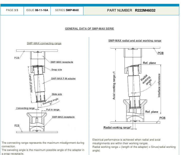
A blind assembly is guaranteed if radial misalignment is smaller than connecting range. Otherwise a manual lead-in is necessary.
