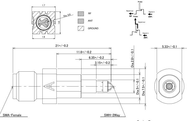
Scale: Free Tolerances Unless Otherwise Specified: +/-0.2 Unit: mm
