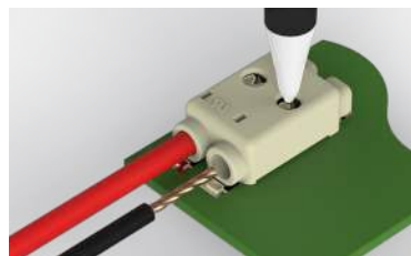
Insert stranded conductors horizontal to printed circuit boards and/or remove both solid and stranded conductors by first depressing the release mechanism with a ball point pen or the tip of any small device. Remove the conductors by pulling horizontal to the printed circuit board.
