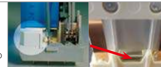
B: Contact circuit 5, 6 Additional physical separator between coil and contacts (for SELV applications)
