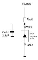
The external resistor Rvdd has to be calculated according to the following formula:
