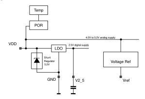
The reference circuit generates an internal supply voltage of 2.5V for the digital logic.
