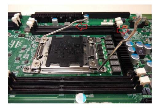
3. Push the CPU socket cover to a fully open position.
