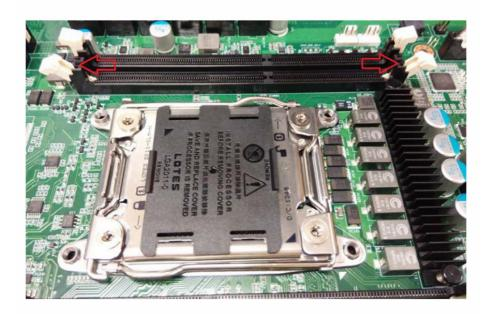
3. Align the memory module with the slot. When inserted properly, the memory slot locking levers lock automatically onto the indentations at the ends of the module. Follow the recommended memory population table to install the other memory modules.
