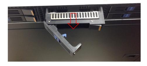
3. Place a hard drive into the drive tray, then use the screws to secure the HDD.
