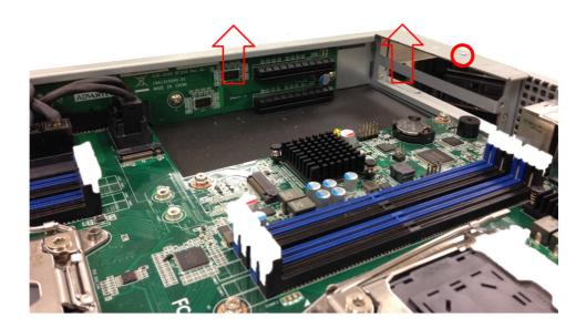
2. Install the expansion card onto the riser card. and screw it onto the riser card bracket.
