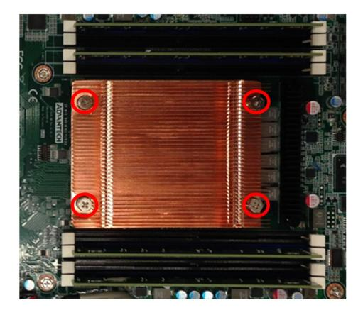
8. Repeat the procedures earlier to install the second processor and heatsink. Now follow the below image for CPU heatsink installation.
