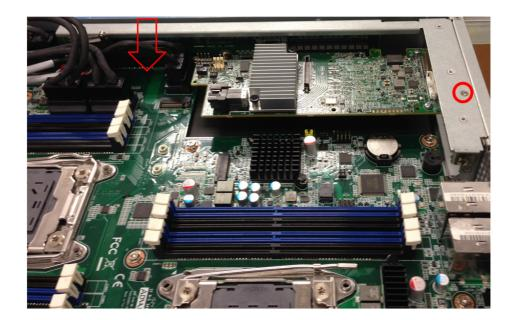
4. Install the mini-SAS HD cable into the expansion card.
