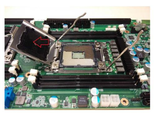
4. Place the CPU into the socket and make sure that the gold arrow is located in the right direction.
