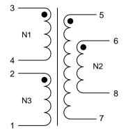
N2 denotes two windings connected in parallel. Terminals 5+6 and 7+8 must be tied as solder bridging is allowed.
