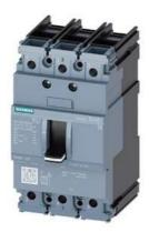
circuit breaker 3VA5 UL frame 125 breaking capacity class M 35kA @ 480 V 3-pole, line protection TM210, FTFM, In=60A overload protection Ir=60A fixed short-circuit protection Ii=10 x In UL489 SB (naval), 50 deg. cel. cable connection on both sides
