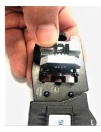
To remover the die set from the hand tool frame loosen thumb Screw (C) completely. Close Ratcheted tool handle one click to reveal the Cap head screw (D). With the opening (E)
