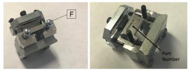
Carefully remove the blade with the springs attached by sliding blade over the alignment pins. When inserting new blade make sure the part number side of the blade is visible before installing cover plate. Re-install cover plate, springs and acorn nuts. Make sure everything moves freely before inserting die set into hand tool frame.
