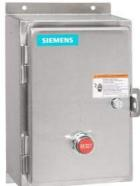
Non-reversing motor starter Size 1 Three phase full voltage Solid-state overload relay OLRelay amp range 10-40a 208VAC 60HZ coil Combination type Water/dust tight non-corrosive
