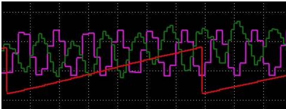
Figure 12. torque effect at no-sinusoidal BEMF
