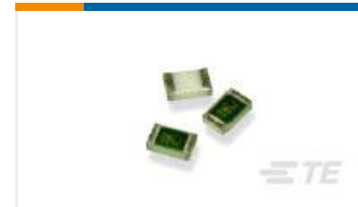
TE Part #3-1879061-4 CPF 0402 200R 0.1% 25PPM 5K RL
