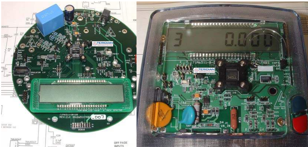
Figure 1-1: Demo Board Versions. 4-layer (left), 2-layer (right)
