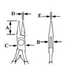
2844D Chain Nose Pliers Serrated Jaw
