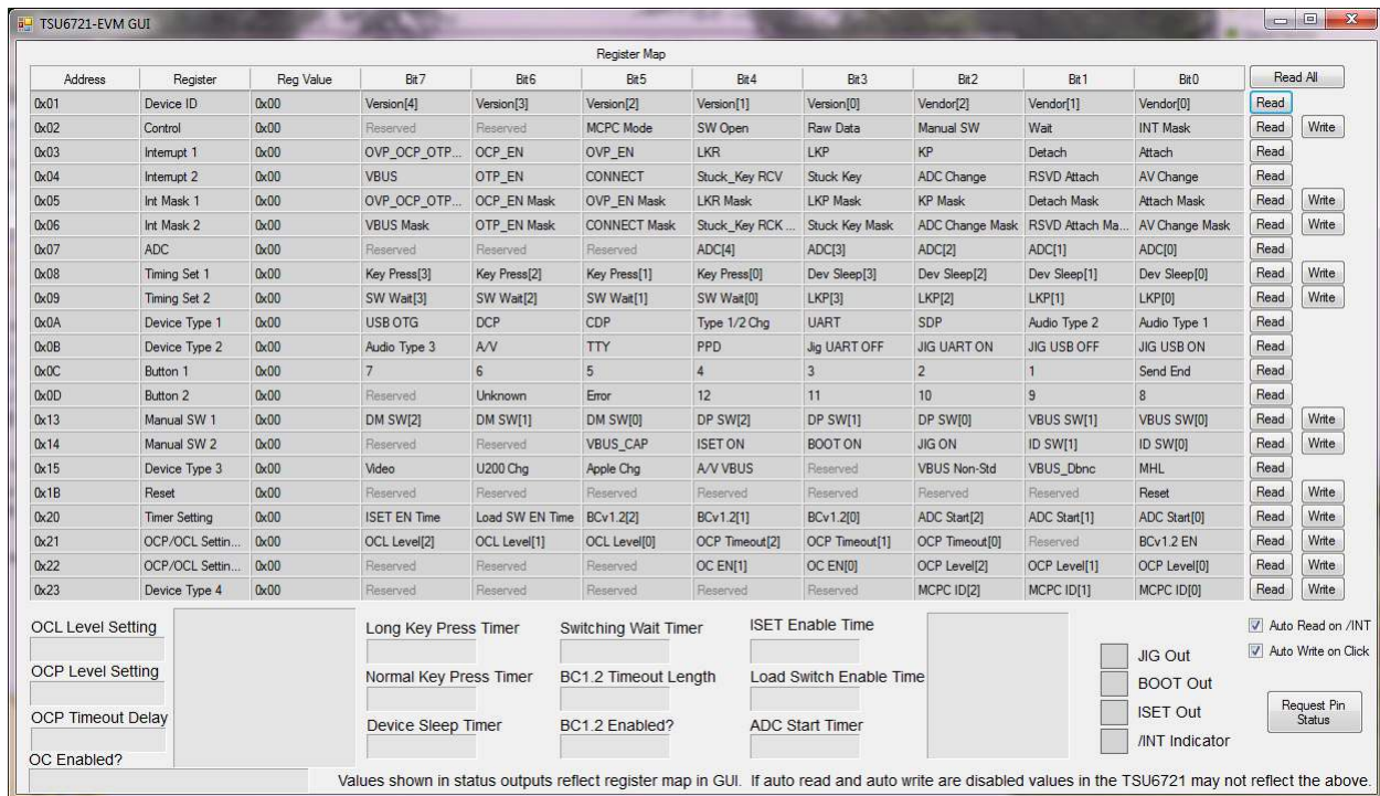
Figure 4. TSU6721EVM GUI Without LaunchPad
