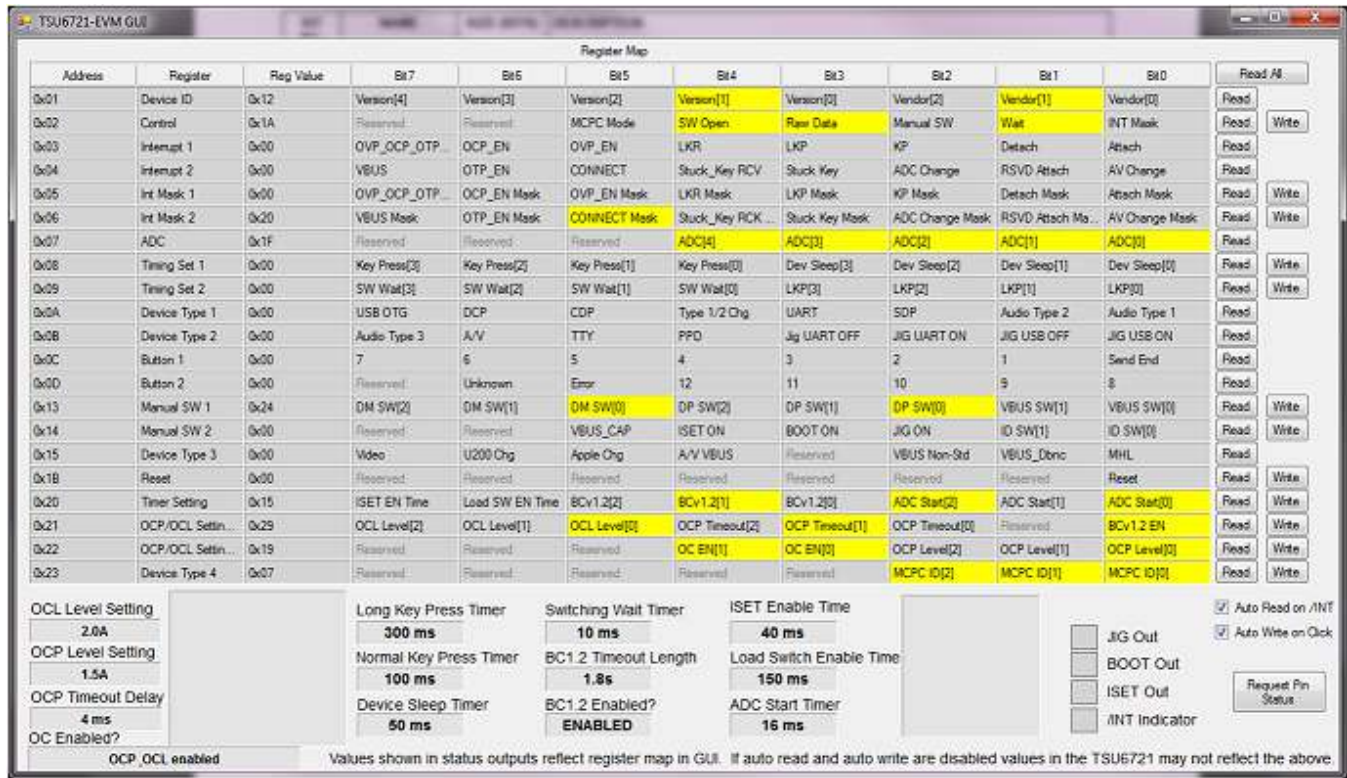
Figure 9. TSU6721EVM GUI Showing Manually Closed DM and DP Switches
