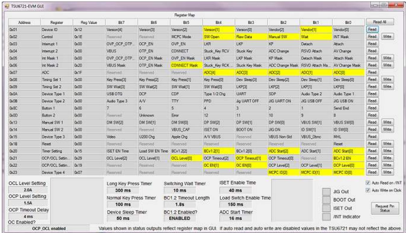
Figure 5. TSU6721EVM GUI After Connecting the LaunchPad to the Computer
