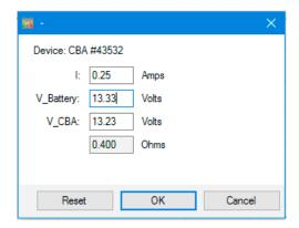
During a high current test there can be a voltage drop between the battery and CBA. This does not affect the current readings. However, it can cause a test to stop earlier than intended. This feature allows for calculating the resistance of the cable and then the software will account for the voltage drop.
