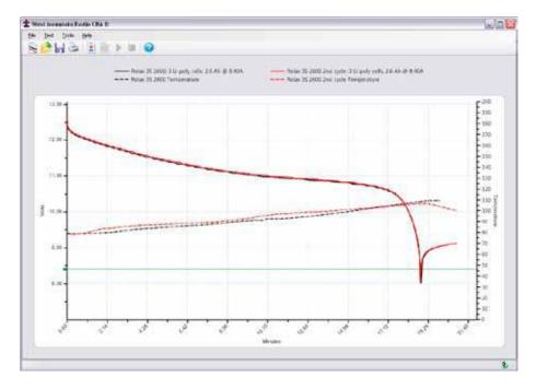
The test will be stopped when the temperature is above the specified threshold or a "Recovery Time" (Discharge Test) can be specified. When the battery reaches the threshold temperature, the test will stop for the given recovery time and then resume. To see the results over time for battery temperature cool down and voltage recovery, use a Voltage versus minutes graph, not Amphrs or Watthrs.
