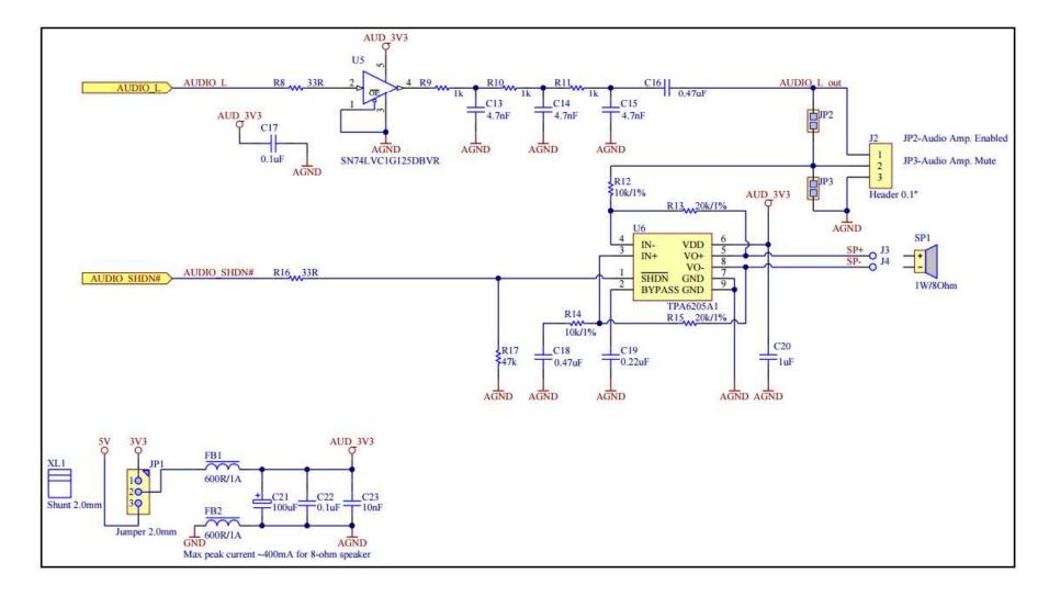
This is a reference schematic from FTDI, which can be used to successfully filter and amplify the audio signals coming from the NHD EVE2 TFT Module.
