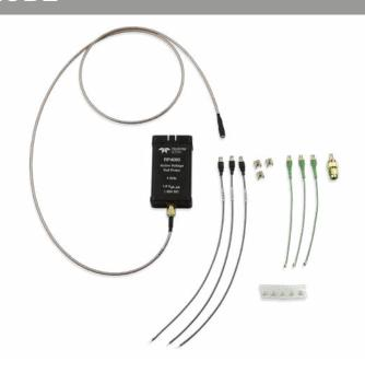
The RP4060 and RP2060 probes are designed specifically to probe low-impedance DC power/voltage rails. Low attenuation means a low-noise view of small signal variations at high frequency, while the probe's built-in offset of up to ±60V enables compensation for the rail's DC voltage. The probe's high DC input impedance eliminates loading of the low-impedance DC rail.
