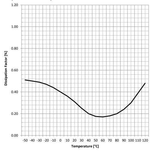
Test Equipment: E4991A or equivalent
