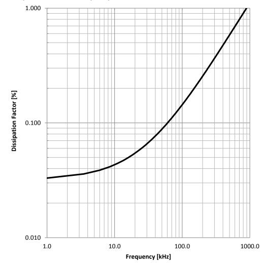
Test Equipment: E4991A or equivalent
