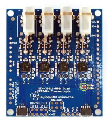
Application: one pair of pull-up resistors are required for proper I2C operation. If multiple breakouts are used together (think Qwiic daisy-chain), it is possible that an excessive amount of resistance can cause bus issues. If this is the case, resistance must be removed from one or more devices. SEN-30011 has cuttable traces on the front side of the board to make this easy.
