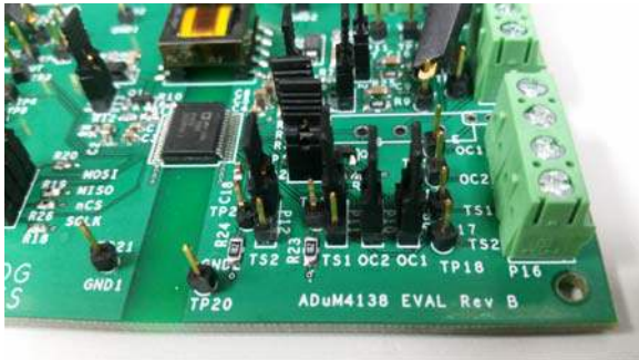
Figure 4. TS1 and TS2 Pins Jumped High (Low Temperature Simulation)
