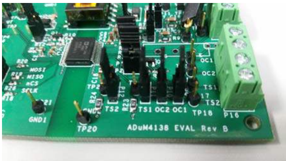
Figure 5. TS1 and TS2 Pins Jumped Low (High Temperature Simulation)
