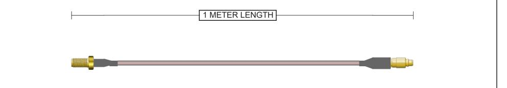
Connector A 132117 SMA Jack Straight Brass Gold + Heatshrink 50 Ohm RG-316 Continuity/Hi-Pot Connector B 262101 MMCX Plug Straight Brass Gold + Heatshrink
