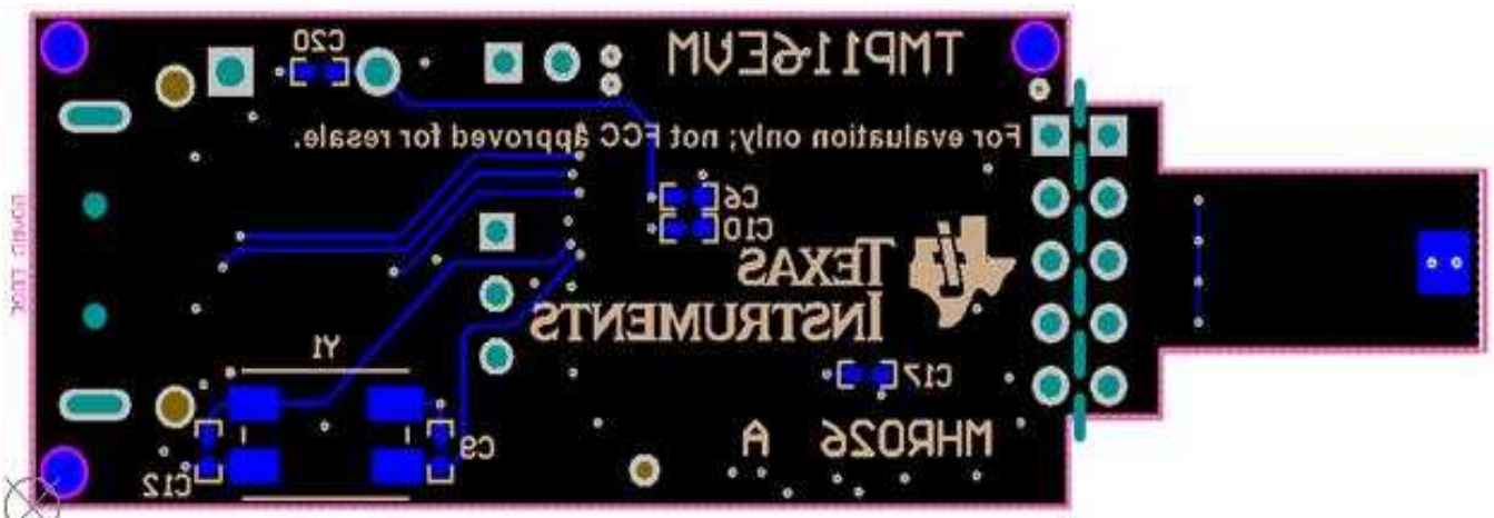
Figure 26. Bottom Assembly Layer
