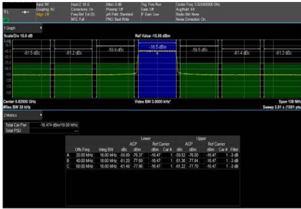
Figure 38. 20 MHz 802.11AC ACLR at 5825.0 MHz
