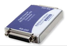
Model 422CEC, RS-232 to RS-422 converter, converts unbalanced RS-232 signals to balanced RS-422 signals. The RS-422 Standard uses a balanced voltage digital interface to allow communications of 90K bits per second on cable lengths of 4000 feet. If this baud rate is exceeded the line length will decrease accordingly. Ten receivers can be connected to any one driver for use in multidrop systems.
