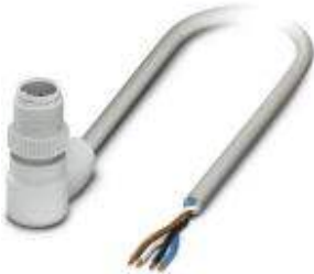
Sensor/Actuator cable, 4-position, PP-EPDM halogen-free, Gray RAL 7035, Plug angled M12, A-coded, on Free cable end, Cable length: 5 m, Hygienic design, with plastic knurl
