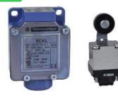
Limit switch, Limit switches XC Standard, XCKL, thermoplastic roller lever, 1NC+1 NO, snap action, 1/2NPT
