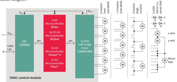
**Example:** The MOTIX<sup>™</sup> TLE94112ES, 12-fold half-bridge, is designed to either drive 6 DC motors up to 0.9 A in parallel mode or 11 DC motors up to 0.9 A in cascaded mode or up to 3 DC motors up to 1.8 A by paralleling two outputs each. The device is sold in a PG-TSDSO-24 package and is pin and function compatible with the 6-, 8-, and 10-fold half-bridge of the TLE94xyz family.
