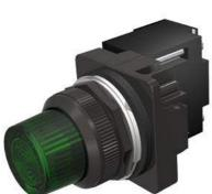
30mm BlackMax, Epoxy Coated Corrosion Resistant Complete Metal Unit Illuminated Indicator Light Full Voltage type, 120V AC/DC LED Lamp, BA9s Glass Lens, Green UL Listed, CSA Certified NEMA 1,3,3R,4,4X,12,13 & Automotive Standards
