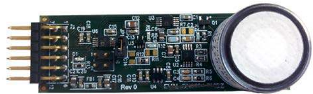
Figure 5. EVAL-CN0357-PMDZ Evaluation Board
