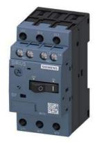
Circuit breaker size S00 for motor protection, CLASS 10 A-release 0.14...0.2 A N-release 2.6 A Screw terminal Standard switching capacity with transverse auxiliary switch 1 NO+1 NC
