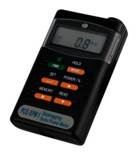
PCE-SPM 1 is a photovoltaic (PV) light meter used to measure solar radiation, solar energy or solar power. The meter's easy-to-read 4-digit LCD screen clearly displays Ptot in  $W/m^2$  or  $BTU/(ft^2 \times h)$ , while the device's auto data memory stores up to 43,000 data sets.
