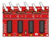
Solder one part at a time. Insert a part into the board, flip the board over, and solder one of the pins. Check to see if the part is still straight. If it isn't, re-melt the joint, and simultaneously straighten up the part. Once it's straight, solder the rest of the pins. You don't have to clip these pins unless you want to.
