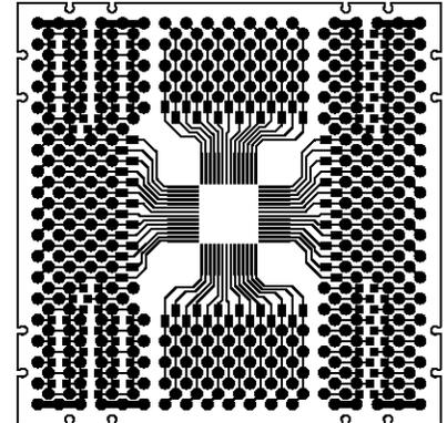
Supports .5mm Pitch 56 Lead QFN devices. A hole in the center of each gives access to a ground or thermal pad on IC.
