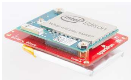
Battery Block Installed
