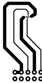
b. 311\text{ }^\circ\text{C/W} when mounted on a minimum pad of 2 oz copper.
