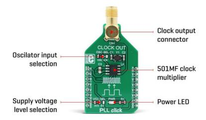
To select the desired multiplication factor, the states of the two input pins S0 and S1, routed to the mikroBUS<sup>™</sup> pins RST and AN, respectively. These pins can be set to a HIGH logic state, LOW logic state, or can be disconnected (by tri-stating the MCU pins). The combination of these pins states will set the PLL click to a specific multiplier. To set the multiplication factor of the PLL click, please consult the multiplication selection table, below.
