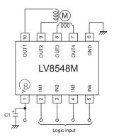
3. Example of applied circuit when connecting it in parallel
