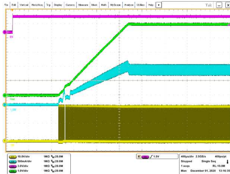
Figure 7. Soft-start phase with I_{OUT} = 1.25\text{ A}
