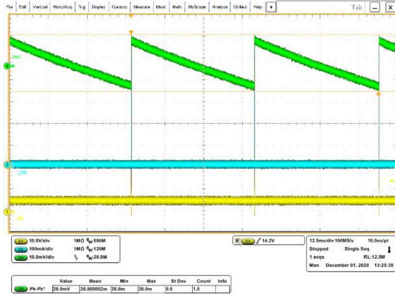
Figure 10. LCM operation at zero load condition (part 1-pulse skipping)
