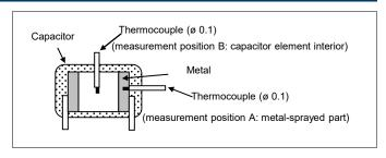
When a capacitor is sent through a high-temperature atmosphere after being subjected to the (flow) soldering process, check the mounting temperature including the temperature of the capacitor in the high-temperature atmosphere.
