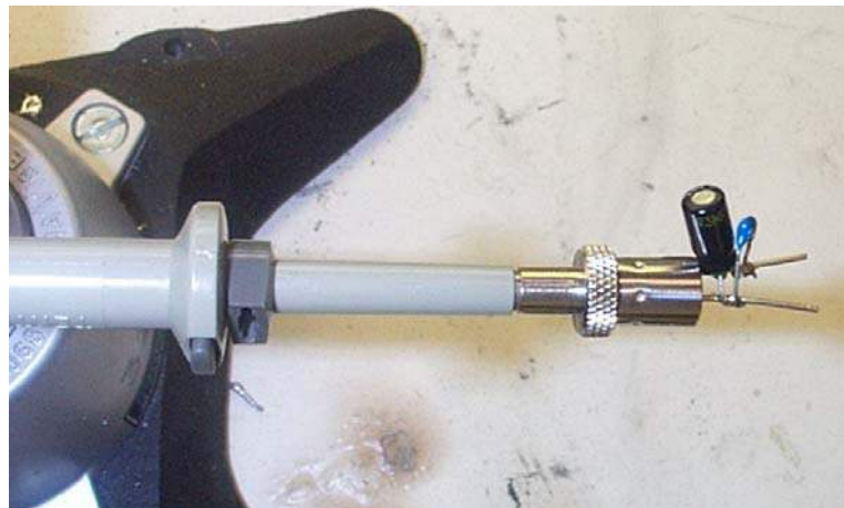
Figure 20 - Oscilloscope Probe with Probe Master 5125BA BNC Adapter (Modified with Wires for Probe Ground for Ripple Measurement, and Two Parallel Decoupling Capacitors Added).
