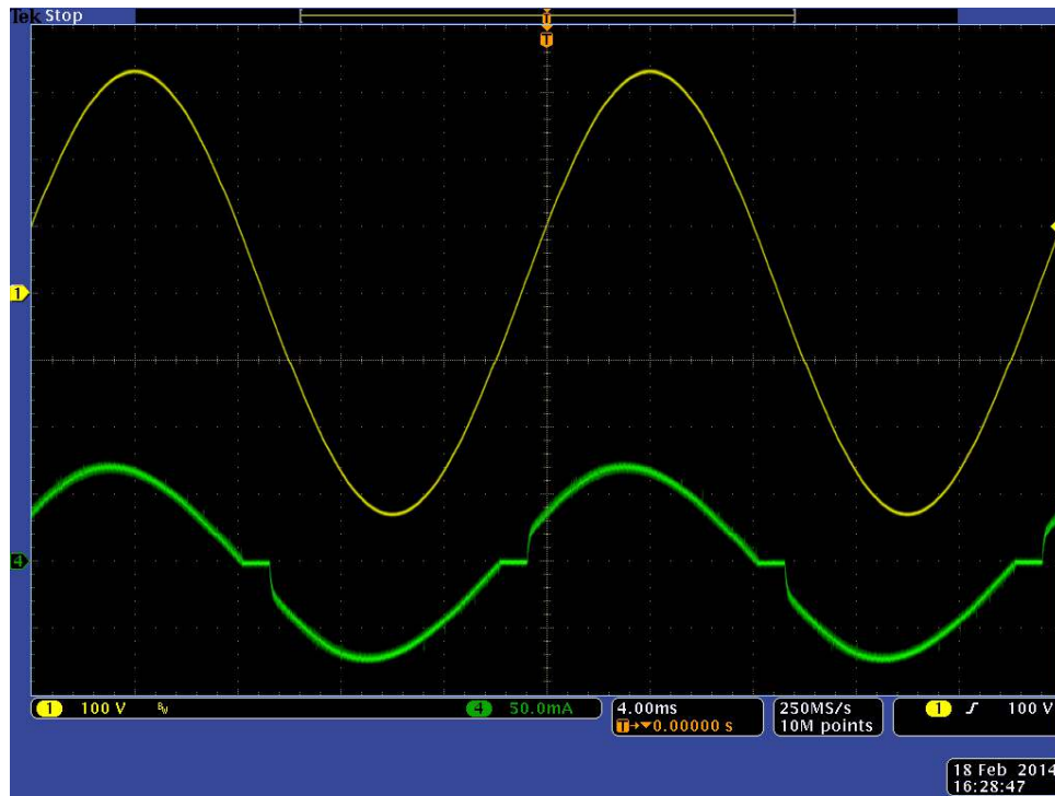
Figure 6. Input Voltage (Top) and Input Current (Bottom)
