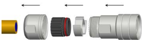
Step 1: Slide parts onto cable
