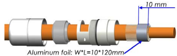
Step 4: Wrap foil over braided shielding
