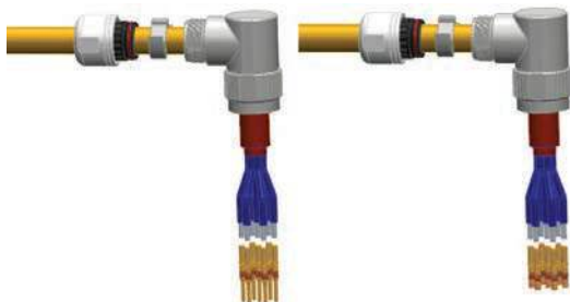
Step 7: Attach contacts to wire leads
