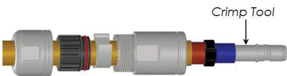
Step 5: Crimp terminal to conductor
