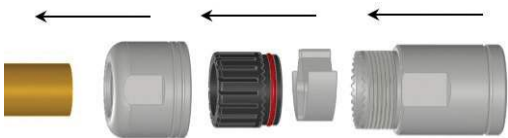
Step 1: Slide parts onto cable
