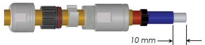
Step 6: Side plug onto crimped terminal assembly
