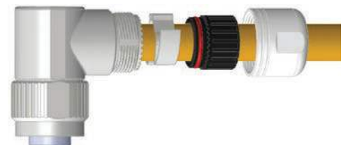
Step 4: Push cable into backshell. Side components onto cable
