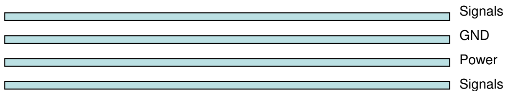
Figure 18: Typical 4-layer PCB construction
