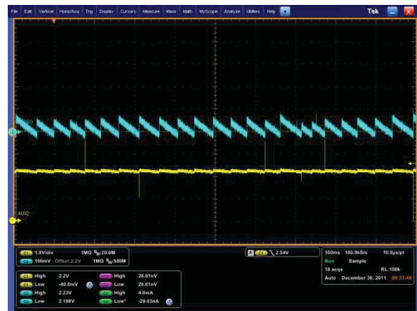
Figure 40. BUCK MINI Output Ripple V IN = 3.6V, V O = 2.5V, I O = 50mA
