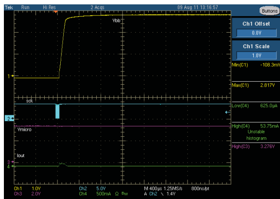
Figure 20. LDO Startup Waveform with I2C Command Ch1: LDO output. Ch 2: I2C SCLK, Ch3: VMICRO, Ch4: VIN current. Startup time is about 200µs.
