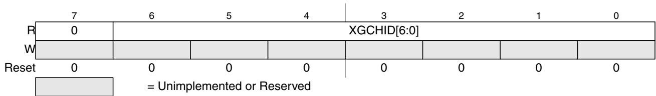
Figure 10-4. XGATE Channel ID Register (XGCHID)
