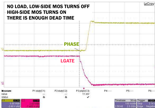
FIGURE 20. GATE DRIVER AND SWITCHING TRANSIENT
