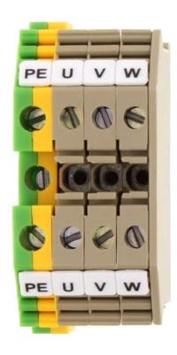
Four-wire motor-connection block, Screw connection, Mounting type:Mounting rail TS 35/7.5 and TS 32, Rated cross-section: 2.5 mm², Colour: Multi-coloured
