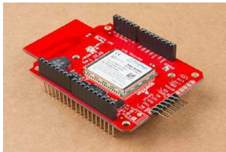
Shield with stackable headers installed.
