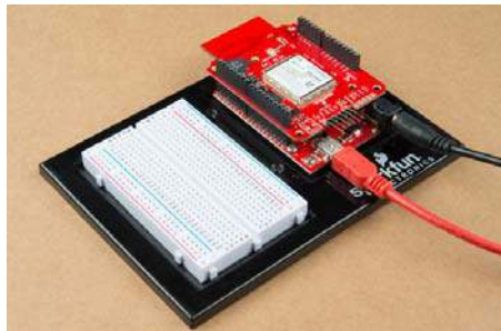
RedBoard with 5V adapter attached
